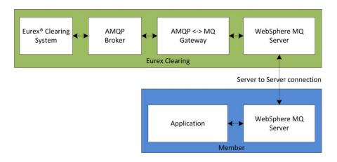
The communication between the Member and Eurex Clearing is established through the WebSphere MQ server-to-server connection. The Eurex Gateway process is responsible for delivering the messages between the AMQP broker and the WebSphere MQ server.
